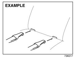
Place the child restraint in the rear seat, feeding the strap hooks through the slots in the seat cushion or the slots in the seatback bottom.
